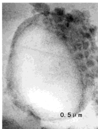
Figure 8. Micrograph of a magnified emulsion-in-emulsion type particle in the ternary blend of PP/PP- g -MAH/PA6 = 35/35/30. (The value 0.5 \mu\text{m} represents the full width of the picture.)
